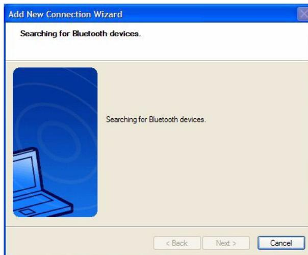
When the Bluetooth device is detected, it is shown in the **Add New Connection Wizard Select a device** window. If multiple devices are detected, each is shown in the window. Select the device to be connected.
