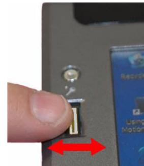
The fingerprint reader also functions as a *scrolling device*; you can move your finger vertically (vertical in relation to the orientation of the Tablet Client) across the scanner to scroll the Tablet Client application within the window.
