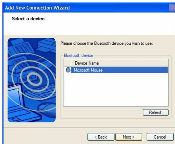
6. Tap **Next** to add the Bluetooth device. The wizard searches for remote device services. The Wizard will display a message that it is connecting and then the passkey number if authentication is required.
