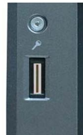
The fingerprint reader also serves as a scrolling device; you can move your finger vertically (from top to bottom) to scroll the cursor within the active application window.
