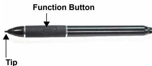
The Motion Digital Pen contains internal electronics that enable you to enter digital ink on the Tablet Client display. The pen is a sensitive, electronic, data-entry device designed in conjunction with the display. The pen includes a user-replaceable tip. The pen
